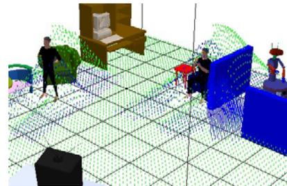
**Figure 10. The “safety”, the “visibility” and the hidden zones” grids. The height of a point corresponds to the cost of that point. The grids were modified to correspond to the results of the user studies.**
